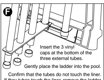
If they tubes touch the liner, remove the ladder from the pool and cut the tubes.
