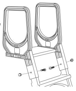
Weight must be added to the bottom of the pool staircase. A coarse gravel or sand may be used. If you use sand, you must seal the sand in a plastic bag to prevent the sand from going into your pool. Simply insert the bags of sand or gravel into the four compartments.
