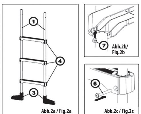
**SCHRITT 3: MONTIEREN SIE DIE KUNSTSTOFFGRIFFE**
