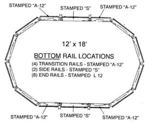
Place bottom rails stamped "S" between the side verticals. Place the bottom rails stamped "A-12" on the outside edge of the side supports as shown above. Place bottom rails stamped "L 12" on the ends of the pool.
