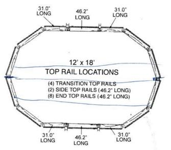
Refer to the diagram above for proper top rail placement.
