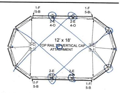
Attach the top rails to the vertical end cap using the hole patterns shown above using #10 x 1/2" screws. Example: On the ends of the pool, attach top rail hole "3" to vertical cap hole "C" and top rail hole "5" to vertical cap hole "I".
